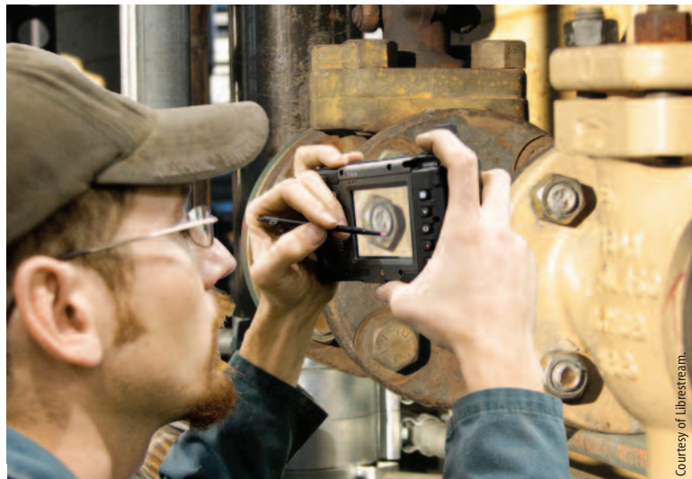
The multi-function camera and communication device allows experts to diagnose problems and lead repairs remotely.
